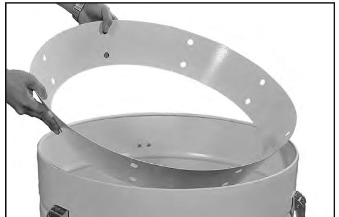
Figure 25. Inserting collection drum vacuum ring.
